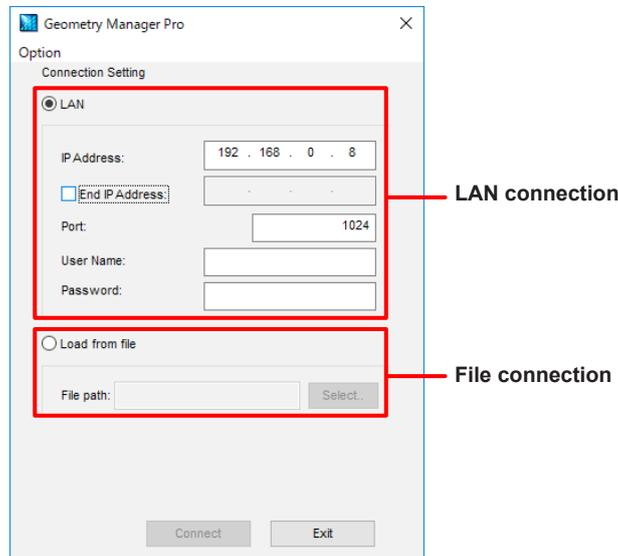
Select [ LAN ] to use a LAN connection for the projector and computer, and select [ Load from file ] to connect by loading a saved file.
